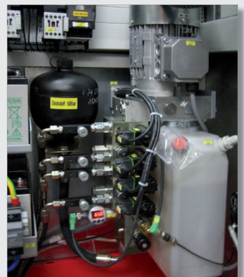
Image 14: Integrated compact hydraulic system
